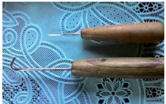
Gantol and tuncek, two indispensable tools for homeworkers to sew shoes, Photo: Dietrich Weinbrenner
