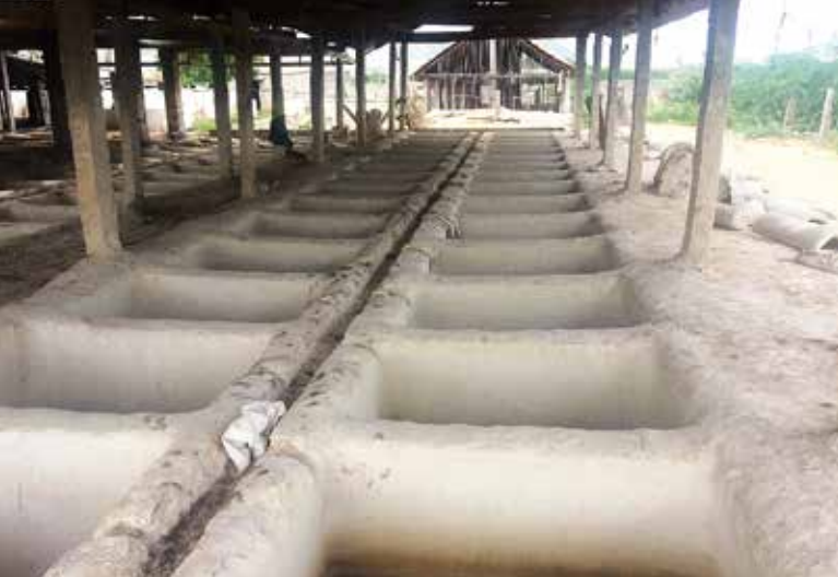
A view of the lime pits in Tannery 1 where the hides are soaked
