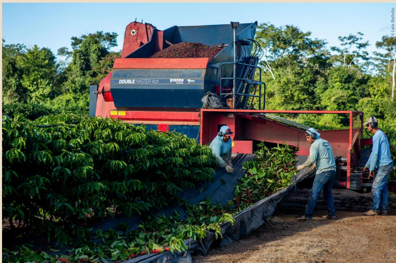
A machine pulls in the coffee plants' harvested branches, chops them up and separates the coffee beans. The workers are exposed to a serious risk of accidents because the required safety distance from the hazardous harvesting machine is not maintained.
